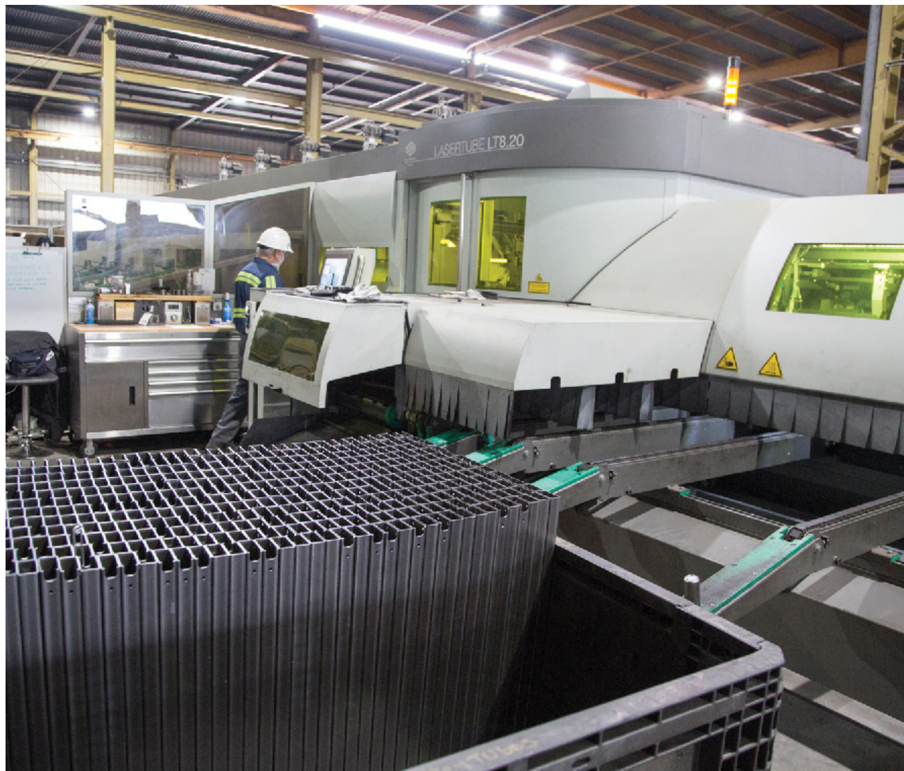
In-house laser processing capabilities were established in 2017 with a Mazak 3D Fabri Gear 400II and BLM LT8.20. »
